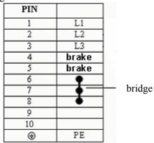
5.1.5.6 Motor connection plug 10-pole with PE socket for star connection with suppressor
